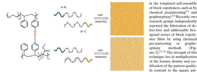
Figure 1. Self-assembly of A-B and B'-C diblock copolymer blends on silicon wafers. The AFM images show that well-ordered square arrays form only when equal numbers of hydrogen-bonding donors (red) and acceptors (blue) are present in the two block copolymers. Reprinted from Ref. [7] with permission; copyright 2008, American Association for the Advancement of Science.
